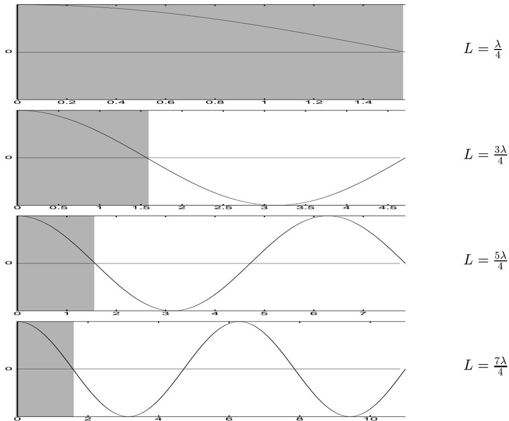
Generally speaking, since each half-period, starting after the first quarter period, begins and ends at 0, we can insert any integral number of half periods and still have a pressure maximum at the closed end of the tube and a pressure minimum at the open end. In other words, odd numbers of quarter wavelengths fit exactly into the length of the tube. We therefore have
