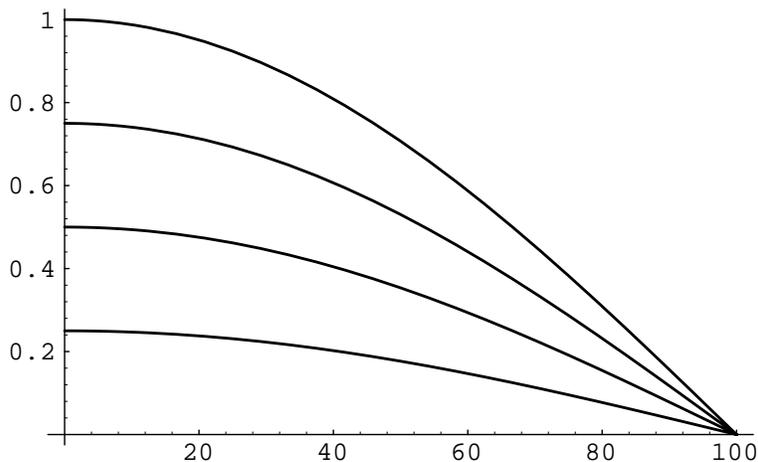
If we scale the ordinate so that the maximum value is at the top, as in the four plots below, we see that the filter characteristics have the same form. That is because we can transform one into the other simply by multiplying by some constant (e.g. by 2.0 to transform the filter with amplitude 0.5 into the filter with amplitude 1.0).
